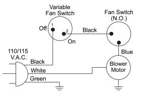
Figure 29 - Blower Wiring Diagram for Thermostat-Controlled Models
